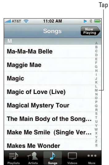
Figure 7-1: Tap the M on the right side of the screen to jump to song titles that begin with M .
